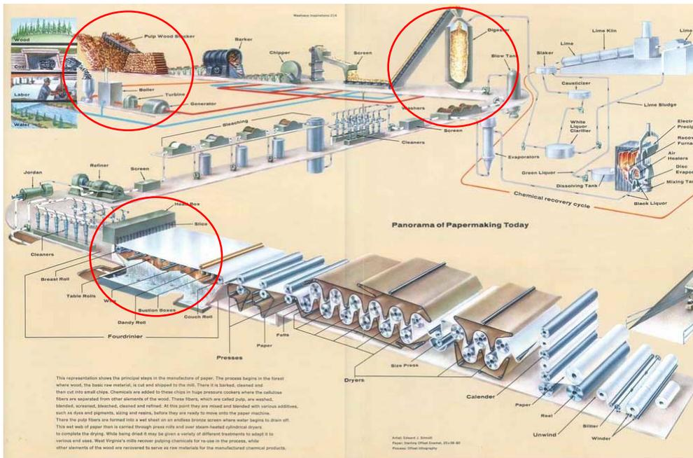
So now when you hear “softwood sulfite” or especially “hardwood kraft,” you know these terms refer to the type of wood, (hardwood or softwood) and method for chemical processing (sulfite or kraft).
