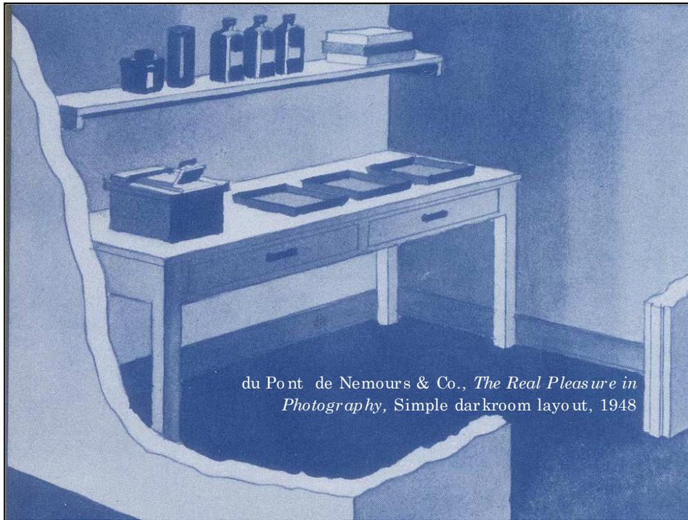
Her next move would be to remove the paper from the printing frame and develop the latent image. Her darkroom would have been laid out almost identically to this depiction from 1948. Here are the three essential trays for the three essential processing chemicals: developer, stop bath and fix.
