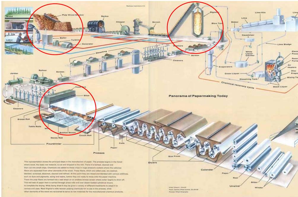
From the Fourdrinier, the paper goes through several drying and pressing steps until it is finally rolled at the end of the process.
