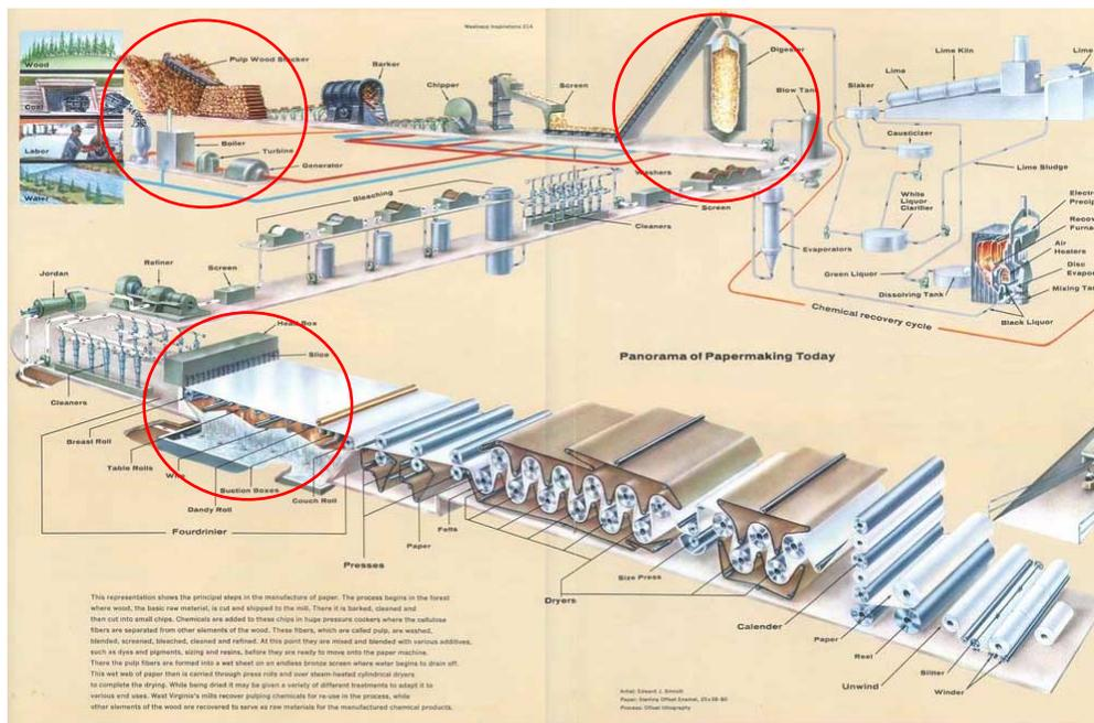
The next important zone is where the wood is physically and chemically converted into pulp.
